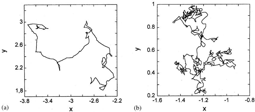
Fig. 10. Typical trajectories of atoms (projection on  $x$ - $y$  plane) at (a)  $T^* = 1.5$  and  $\rho^* = 0.2$ , (b)  $T^* = 1.5$  and  $\rho^* = 0.8$ .
