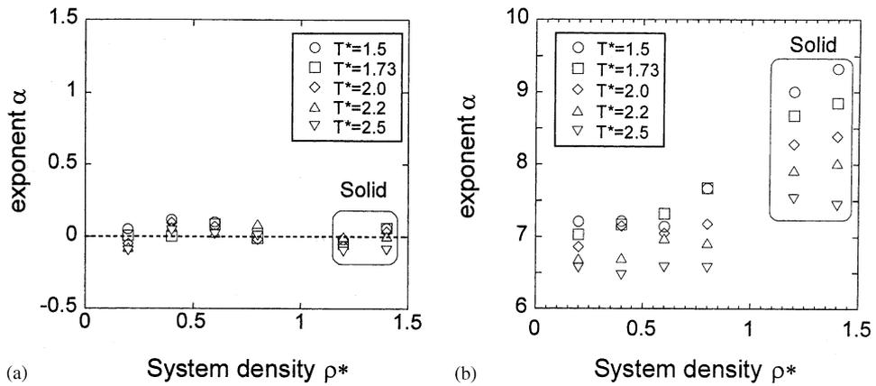
Fig. 5. Pressure power spectrum  $\alpha$  exponent as a function of system temperature and system density (a) low-frequency domain, (b) high-frequency domain.
