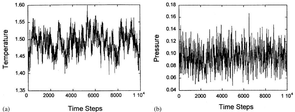
Fig. 1. Time series emanating from MD simulations at system (average) temperature  $T^* = 1.5$  and  $\rho^* = 0.2$ . (a) instantaneous temperature, (b) instantaneous pressure.
